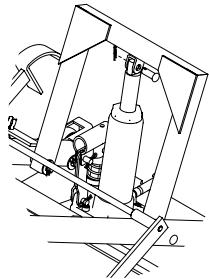
Figure 4: Inserting Bottle Jack Pin.
