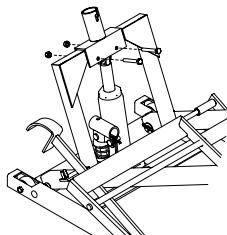
Figure 6: Handle Yoke assembly.
