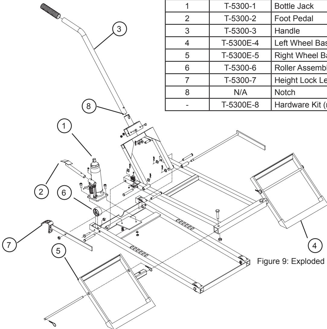
**⚠ WARNING:** The Lift Handle is used to operate the Bottle Jack Release Valve. Exercise caution when adjusting the Release Valve raise and lower load slowly and carefully.
